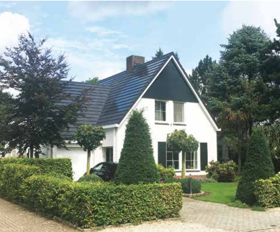
The integrated PV Solar Tiles used with Crest Planum roof tiles in Onyx black
